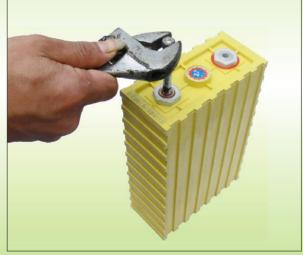
用專用開螺紋工具重新開牙 Please remake the screw thread with special to
