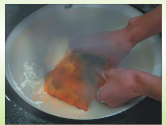
將冒烟燃燒的電池浸入水中 Put the burning battery into water
