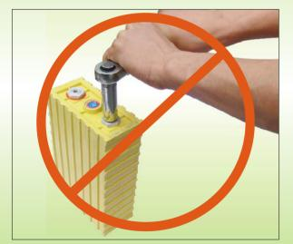
電池極柱中間螺絲滑牙 Terminal screw thread damaged and become less crowded
